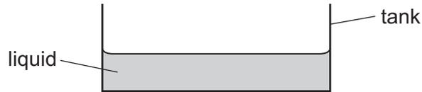
The base of the tank is rectangular and has dimensions 0.20 m by 0.50 m.
